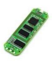
The multi-interface and multi-technology RFID module "AIO" offers an extreme level of flexibility.
