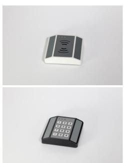
The new multi-functional and multi-technology RFID reader MCR\_Flex gets its name from its extreme flexibility in applications, suited for use with transponders in all common 13,56 MHz technologies. This universal application possibility offers enormous advantages compared to other readers supporting just one technology.
