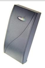
The PREMIUM-MF type is a contactless reader device in the frequency range of 13,56 MHz. This reader will read the unique ID number of a Mifare® card and output that code in any of many user selectable formats. Due to the fully potted housing, the reader can be installed both indoors and outdoors.
