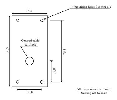
If the mounting plate is used the reader cable may be brought out of one of four exit points on the mounting plate: top, bottom, left or right. This enables the cable to be run on the surface of the wall.
