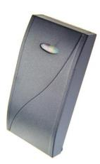
The PREMIUM-MFS is a Mifare reader that is user configurable to read data from a designated sector using a designated key. As this data cannot be copied from the Mifare card, it provides a secure card reader. Card readers are supplied in a factory reset state and are programmed using a configuration card. On first time power-up the reader LED's indicate that the reader needs to be configured.
